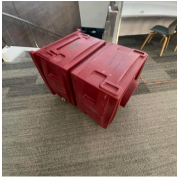
35. Third Floor - Main Area: Equipment On-site 1 - Air Scrubber
